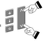
■ <u>STANDARD THERMOSTAT</u> - While in standard thermostat setting, the transmitter will turn the burner on and off to achieve the target temperature (see below). To adjust the target temperature, press the up and down buttons until a suitable temperature is achieved.
