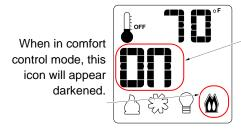
This is the comfort control read-out. Use the up button to turn on, down button to turn off (2 settings).
